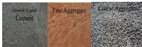
Fig:View of cement, fine aggregate and coarse aggregate
