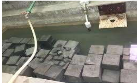
Fig. view of curing
