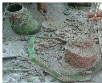
Fig. Testing of slump cone
