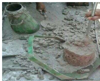
Fig. Testing of slump cone
