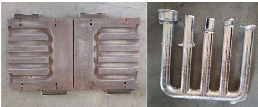
Fig.2 (a) Metallic Die (b) Casting after solidification
