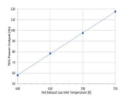
Maximum power generated by a TEM can be calculated as the ratio of OCB to the 4 times of the internal resistance and it was defined as an UDF (user defined function, which was developed and defined in the ANSYS fluent program to predict the electrical power output) during the simulation.
