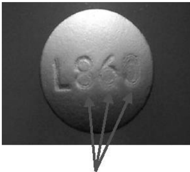
Fig.30: Erosion of the logo on the tablet
