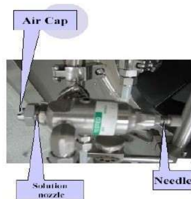
Fig.15: Air cap, solution nozzle and needle of the spray gun for film coating
