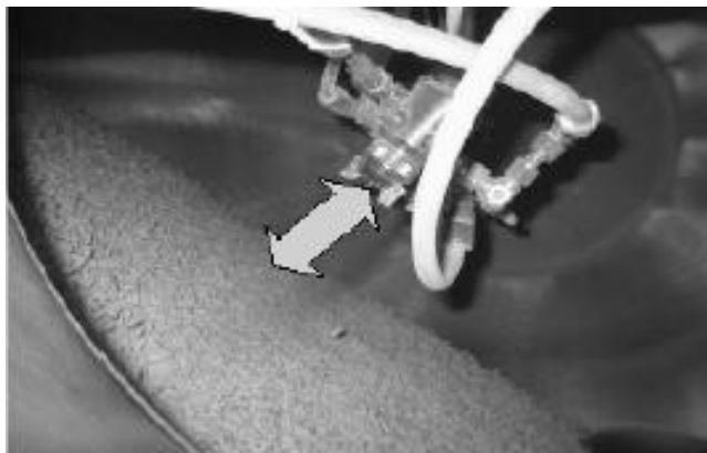
Fig.21: Gun to bed distance
